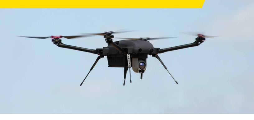
Part of the Robotic Autonomous combat Solution (RAS), the Magni-X VTOL (vertical takeoff and landing) micro-UAS is a fully autonomous military multi-rotor platform with a sophisticated close-range observation system. Suited for a wide range of missions and applications, the Magni-X is specially designed for Short Range Reconnaissance (SRR) and for the urban arena, providing day and night intelligence imagery powered by advanced AI algorithms for tactical combat units.
