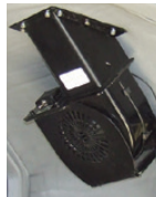
Firing Gas Disposal Blowers
