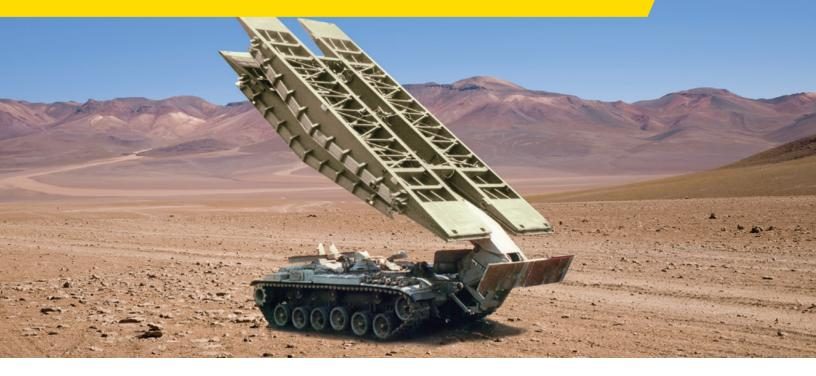
The Tandem Assault Crossing System (TACS) is an assault bridging system with multiple-gap-crossing capability. The system enables enhanced maneuverability on the battlefield, providing armed forces with an immediate solution to overcome obstacles to forward progress. The system enables operation in mountain terrain, including over deliberate road craters, and offers multiple obstacle capability. The TACS ensures high survivability and redundancy.
