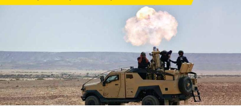
Elbit Systems' SPEAR is a fully autonomous, vehicle-mounted 120mm soft recoil mortar system for high-mobility platforms. SPEAR delivers effective fire support by combining the flexibility and effectiveness of accurate mortar firepower with exceptional tactical mobility. The mortar is a derivative of the CARDOM battle-proven mortar system - more than 1,000 systems extensively used by the US Army, NATO, Israeli Defense Forces (IDF) and others.
