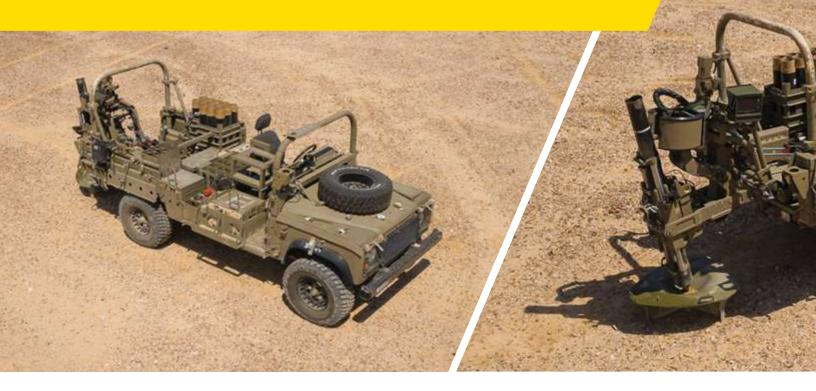
A fully autonomous, computerized, mounted mortar system with the dimensions and weight of a small carrier vehicle, the SLING is adaptable to a wide range of high mobility platforms. The rapidly deployed 120mm mortar system enables quick response and enhanced survivability, in and out of action within 30 - 60 seconds, with shoot & scoot capabilities. SLING is easily operated by a 2 - 4 person crew.
