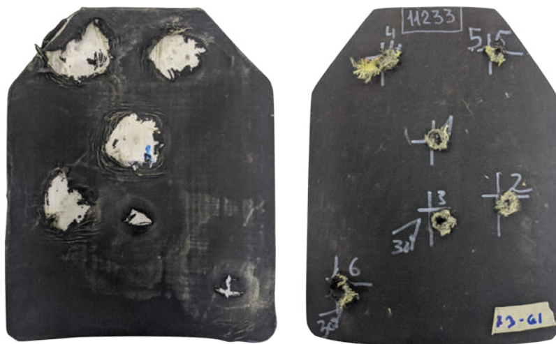
Standalone hard ballistic plate with 6 hits of armor piercing AK-47 7.62x39 API-BZ bullets, including 3 shots 35mm from the edge of the plate. All shots were completely stopped by the plate.
