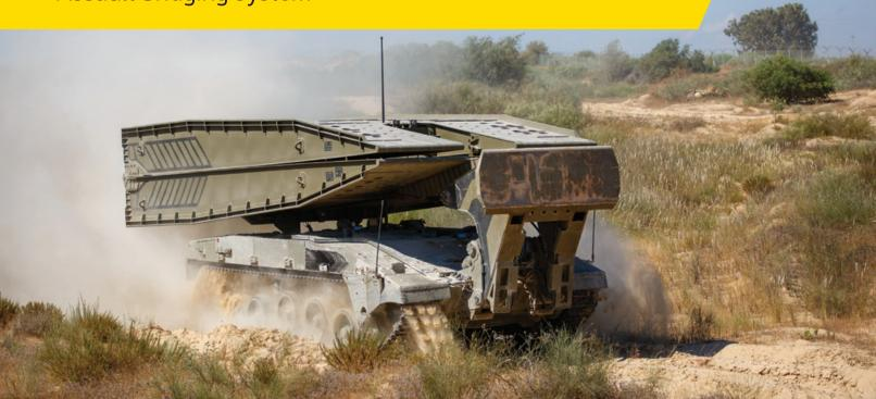
The Armored Vehicle-Launched Bridge (AVLB) assault bridging system provides armed forces with enhanced mobility and maneuverability on the battlefield, enabling rapid and efficient gap crossing. Featuring multiple STANAG protection levels, the AVLB offers an optimal solution for various combat scenarios. The system can be adapted to customer needs and fleet.
