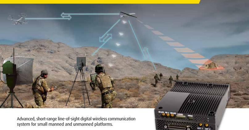
With an operational range of up to 70 km, the StarLite SR is an advanced line-of-sight (LOS) short-range digital wireless communication system for small manned and unmanned platforms. Supporting several data rates of up to 8Mbps, the system's next-generation technology ensures smooth SD/HD video and audio or data from the payload to the ground station even in harsh conditions, in the air, at sea or on land.
