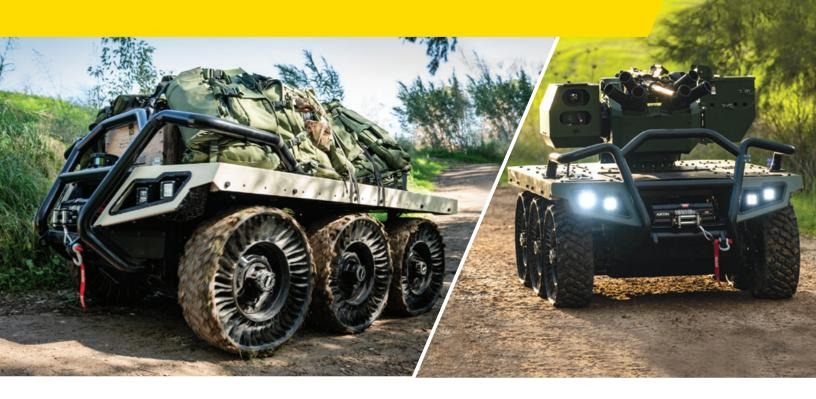
Part of the Robotic Autonomous combat Solution (RAS), the ROOK high mobility 6x6 unmanned ground vehicle (UGV) with all-terrain maneuverability is suitable for close and long-range operations under extreme conditions. Designed to carry heavy payloads, the multipurpose robotic UGV can perform a wide range of urban warfare, battalion maneuvers and border protection missions while increasing front-line effectiveness and survivability.
