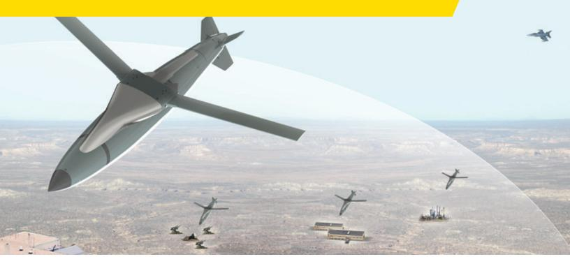
The Range Extension and Smart Tail (REST) guidance kit for general purpose warheads, upgrades the weapons capability of any aircraft to deliver extended range precision strikes. The system incorporates a smart tail for navigation and upper wings for range extension.
