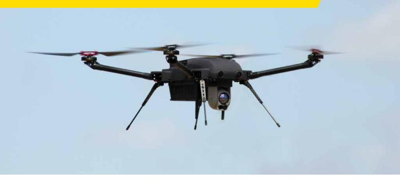
Part of the Robotic Autonomous combat Solution (RAS), the Magni-X VTOL (vertical takeoff and landing) micro-UAS is a fully autonomous military multi-rotor platform with a sophisticated close-range observation system. Suited for a wide range of missions and applications, the Magni-X is specially designed for Short Range Reconnaissance (SRR) and for the urban arena, providing day and night intelligence imagery powered by advanced AI algorithms for tactical combat units.
