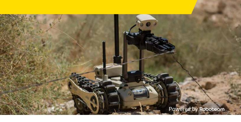
The MTGR (Micro Tactical Ground Robot) platform is a unique and lightweight all-terrain tactical robot with high maneuverability indoors and outdoors. The MTGR is specially designed to support military, law enforcement and public safety units in various combat situations around the globe. Perfect for explosive ordinance disposal (EOD), urban warfare, special operations or public safety missions, the MTGR dominates the unknown.
