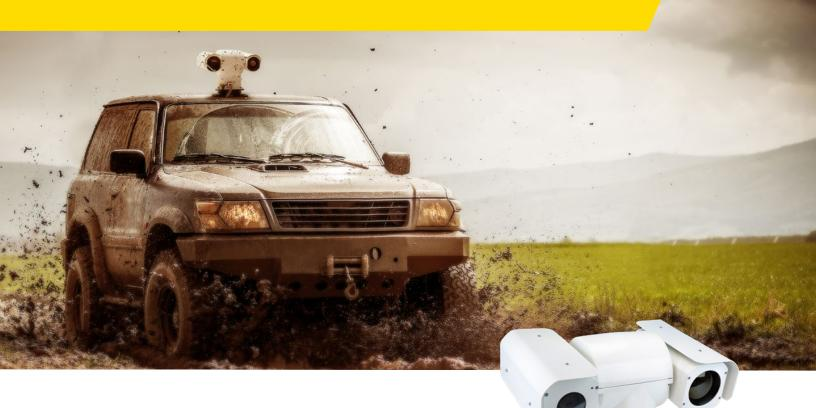
Mobile Surveillance System is a compact and lightweight 24/7, thermal and visible multi-sensor observation system developed for security applications. It allows mid-range observation and detection using advanced thermal imaging and HD CMOS technology.
