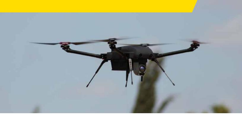
The Magni-X VTOL (vertical takeoff and landing) Micro-UAS is a military fully autonomous multi-rotor platform with the most advanced close-range observation system. Though suited for a wide range of missions and applications, the Magni-X is specially designed for Short Range Reconnaissance (SRR) and for the urban arena, providing day and night intelligence imagery powered by advanced AI algorithms for tactical combat units.
