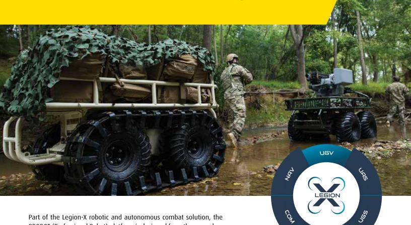
Part of the Legion-X robotic and autonomous combat solution, the PROBOT (Professional Robot) platform is designed from the ground up as an autonomous, robust, lightweight tactical support vehicle with high mobility and all-terrain maneuverability in urban and rural environments. Featuring a common all-electric chassis with a very low thermal and acoustic signature, PROBOT can carry heavy payloads and integrate in logistics, medevac, CBRNE, ISR and special operations.
