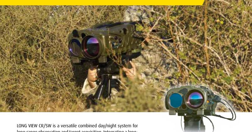
long-range observation and target acquisition. Integrating a long-range zoom thermal, day and SWIR (optional) channels, eyesafe laser rangefinder, GPS and magnetic compass and mounted on a tripod or P&T, LONG VIEW CR is an outstanding tool for acquiring targets and engaging fire from long ranges.
