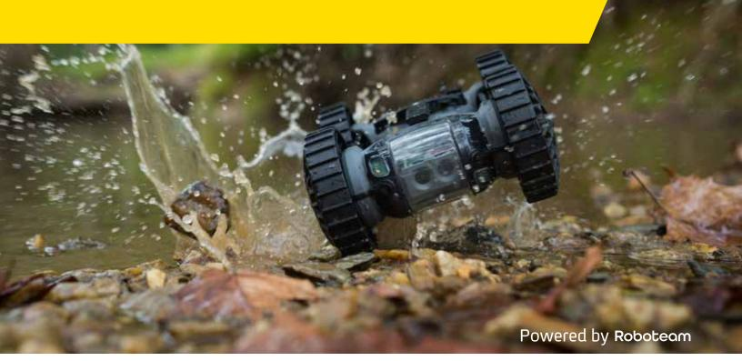
The IRIS (Individual Robotic Intelligence System) is a miniature, rapidly deployable, ruggedized, hand-carried, unmanned system. The system is designed to support units such as SWAT, public safety, military and law enforcement. The IRIS can enter small and confined spaces, above or underground, to explore hazardous areas while relaying intelligence and reconnaissance information in real-time.
