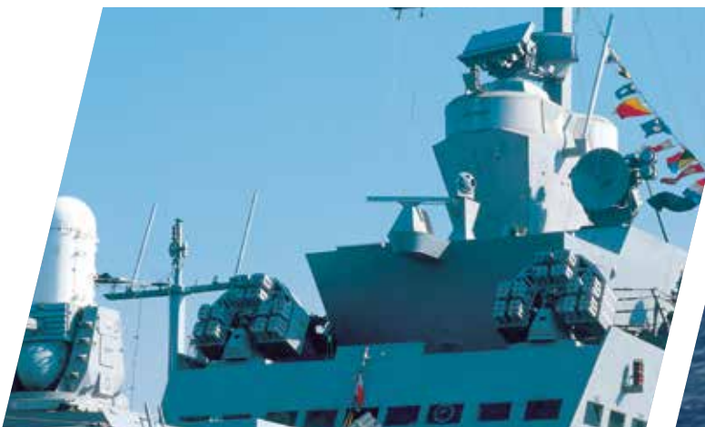
DESEVER – Decoy Control and Launching System – responds simultaneously to multiple threats by delivering various payloads at accurate time intervals, according to specified anti-missile doctrines and guidelines.
