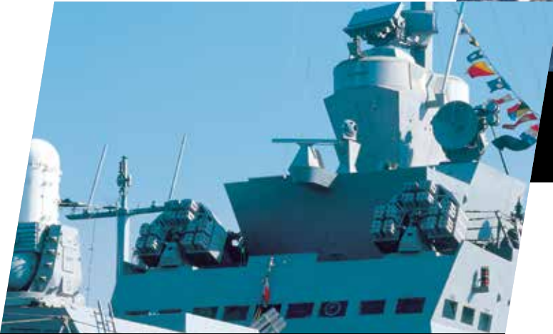
DESEAVR – Decoy Control and Launching System – responds simultaneously to multiple threats by delivering various payloads at accurate time intervals, according to specified anti-missile doctrines and guidelines.
