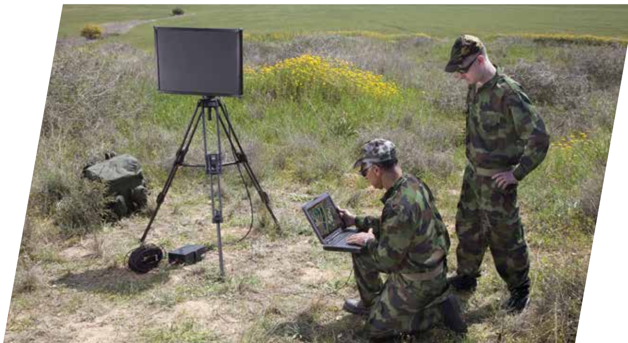
FOXTRACK™ – a portable Ground Surveillance Radar System – is a lightweight, compact, man-portable radar carried by two operators soldiers, special operations forces or security personnel.
