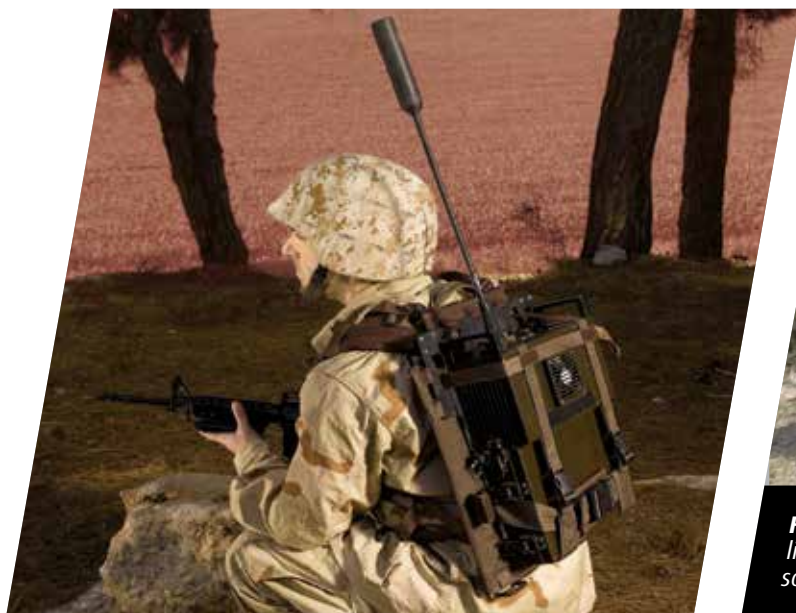
Miniature Reactive Jammer (MRJ) – An RF-based family of systems that effectively counters improvised explosive devices reactively, actively or both simultaneously, and is offered in man-pack, vehicle-mounted and portable rolling case options for use by military, HLS and police forces.
