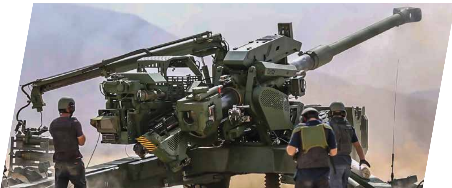
ATHOS is a long-range 155mm/52 caliber autonomous towed howitzer capable of a range greater than 40km.
