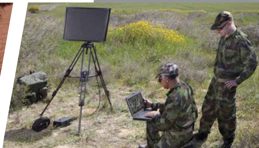
FOXTRACK™ is a portable Ground Surveillance Radar system that is lightweight, compact, man-portable and can be carried by two operators, soldiers, special operations forces or security personnel.
