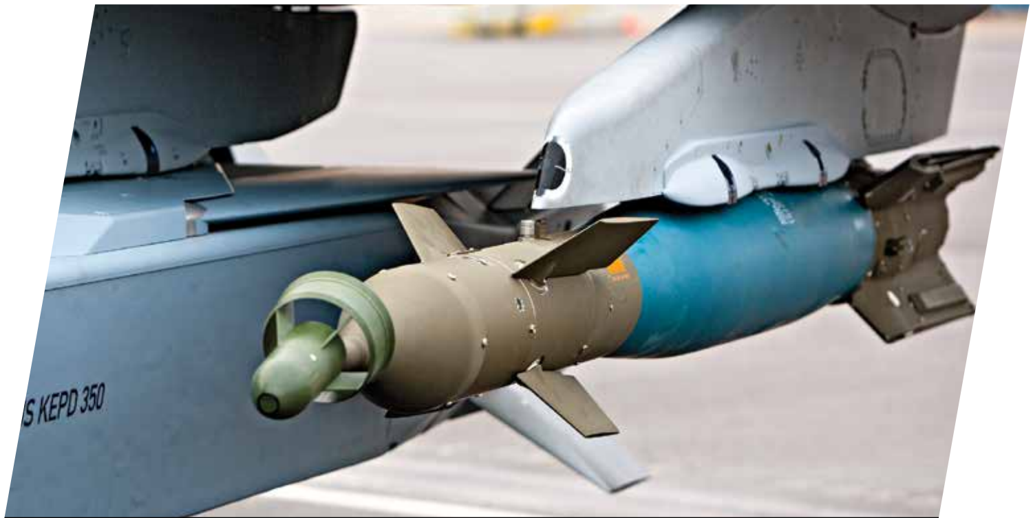
Lizard™ – a modular guidance kit for precision strike capabilities.
