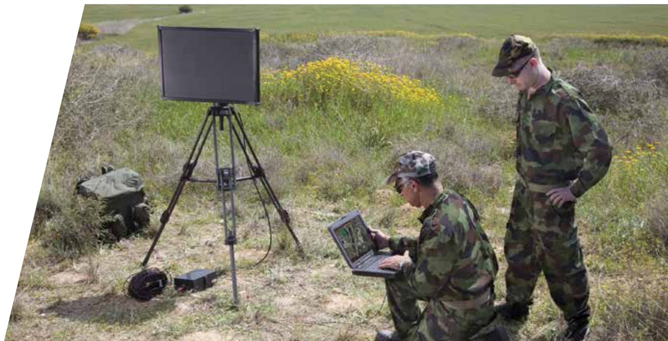
FOXTRACK™ – a portable Ground Surveillance Radar System that is a lightweight, compact, man-portable radar carried by two operators, soldiers, special operations forces or security personnel.
