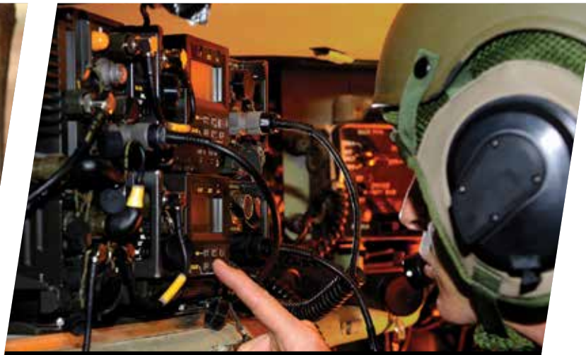
CNR-9000HDR – Combat IP radio, advanced multi-mode VHF/FM COMSEC/ECCM radio system for superior voice and high-speed data communications.
