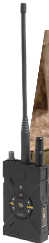
PNR-1000 is the latest in a line of innovative personal network radios (PNR) providing combat-proven voice, data and video communications solutions to the dismounted soldier.
