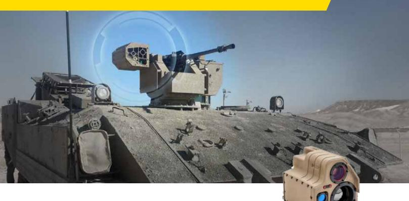
As an advanced firing system, Dragon Eye allows target detection, recognition and identification under extreme visibility and environmental conditions. Dragon Eye can quickly spot targets in both day and night, using multi-sensor cameras installed on armored personnel carriers (APC).
