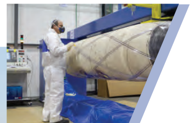
330 Gallon filament winding process
