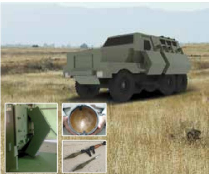
The Breakwater hybrid protection system is based on passive and active armor technologies, designed to minimize the risk of injuring dismounted troops and of collateral damage to non-combatants. The complete armor solution provides a high level of protection against IEDs explosively formed penetrators (EFP) and RPG-7 anti-tank warheads. The shape is optimized to achieve the ideal balance of performance to protect against EFPs and RPGs.
