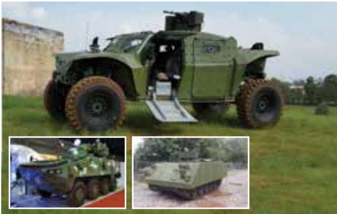
The experience gained with heavy main battle tank (MBT) armor protection has been leveraged and implemented on several lighter platforms. Protection kits developed for the IDF and other customers include systems for the M113 APC and wheeled platforms, such as the CombatGuard, and a tailor-made solution for ICV (8x8 Infantry Carrying Vehicle).
