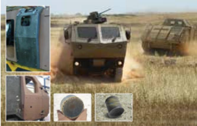
Iron Wall is a combat-proven innovative passive ballistic structure capable of defeating medium IED threats, such as explosive flyer plates EFPs and steel-ball charge focus fragments SFFs. The solution provides passive add-on armor comprising a combination of composites and metals. The protection system is compatible with medium and light platforms (tracked or wheeled APCs).
