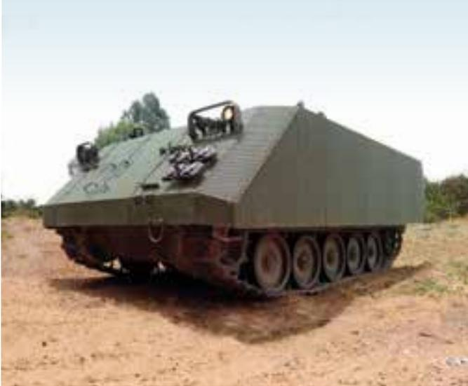
TOGA is an add-on armored solution composed of specially perforated steel plates. The cost-effective solution offers low-weight protection for APCs against AP bullets, and artillery and shell fragments. The add-on armor provides high-level ballistic protection (350% efficiency) by deflecting the bullets' trajectory and protects against RPGs by reducing the dispersion. TOGA is type-qualified and fielded by the IDF and other forces worldwide.
