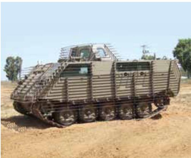
The Urban Fighter suite for M113 provides all-round visibility, advanced firing capabilities and high-level passive armor protection against IEDs, RPG (SLAT), and 14.5mm AP bullets. The vehicle can carry nine fighters with full combat gear.
