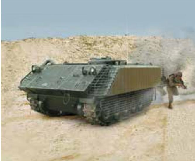
The light vehicle armor system (LVAS) is based on modules that are easily replaceable in the field, providing low weight protection against multiple threats: RPG-7 warheads (perpendicular hits), IED and artillery fragments, 7.62mm and 14.5mm AP bullets. With optimal explosive and metallic contents, the add-on hybrid (passive and reactive) modular armor system is a reliable and safe solution for APCs crew and deployed troops.
