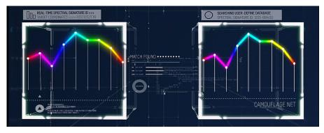
Using Module CU on a platform, a search is made for materials in real-time, comparing them to the sample stored in the database. When a match is discovered, the CU Module alerts the user. Comparisons can also be made on anomalies.
